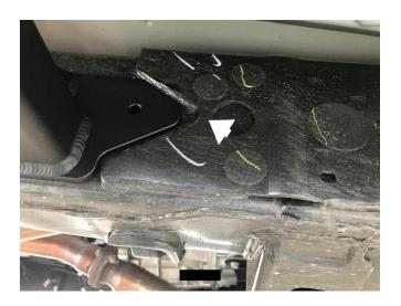
7. Use supplied hardware with small washers on the face and large washers on the rear where there are large round or square holes in the factory frame rail. Install nuts but do not tighten. Use at least 6 supplied new bolts per side. Removal of the white plastic line clamps is necessary.
