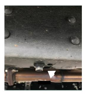
Place slider on frame rail with point facing forwards and re-install 14mm crossmember bolt on bottom loosely to hold slider in place (use supplied 3/8 hardware for 4-door longbox models).
