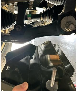
5. Next install the smaller 5/16" bolt in the smaller hole closest to the wheel, with a 3/8" spacer between the skid plate and the control arm. Again, loosely install the washer and nylock nut on top of the control arm.
