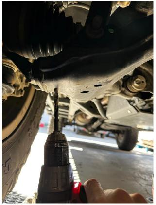
3. Gather a control arm skid plate and half of the supplied hardware. Passenger side shown.
