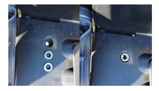
5. Place the bracket and install with the two factory bolts in the floor of the bed loosely.
