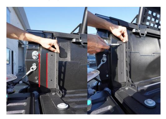
7. Remove the bracket and use a center punch to mark the holes.
