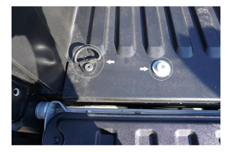
3. The factory tie-down bolt will be disassembled and only the bolt, spacer, and lock washer will be used when re-installed.
