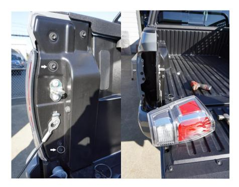
2. Remove two Torx bolts from bed – keep these as they will be re-installed.
