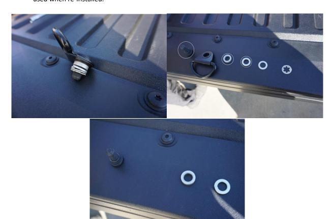
4. Put the spacer and lock washer back in the hole they were in with the lock washer on top. Put the bracket in place on top of these.
