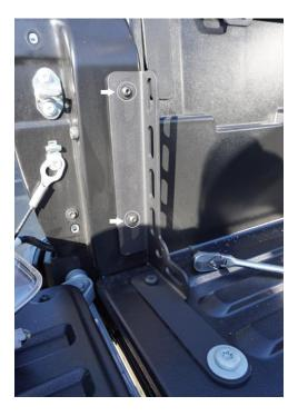
11. Install the backing plate (in tail light space) using the stainless washers and nuts.
