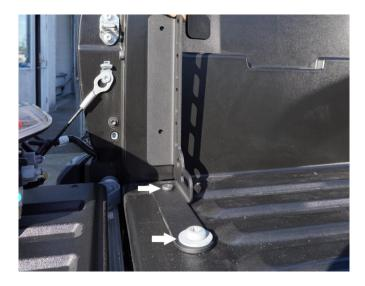
6. Hold bracket in place so that it is parallel with the edge of the box and mark the placement of the two side holes with a pen/pencil.
