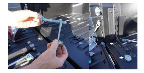
10. Put never-seize (or blue Loctite) on the 5/16" bolts and install with the black flat washer through the holes on the side of the bracket and through the box.
