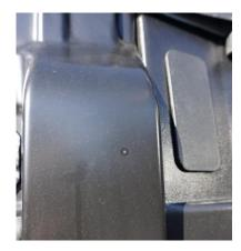
8. Drill the two holes to 3/8" – using a step drill bit will give best results.
