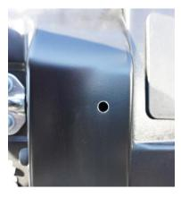
9. Put never-seize (or blue Loctite) on the factory bolts and reinstall with the bracket; do not tighten these bolts **yet**.
