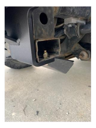
8. Install supplied 5/16" bolts and fender washers to hold plastic bumper front and inner fender together on passenger and driver side.
