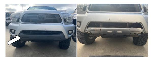
3. Carefully trim the center section of the plastic bumper using an angle grinder or reciprocating saw to allow access to the aluminum crashbar. These cuts will be cleaned up later.
