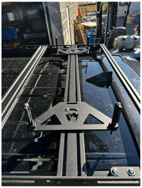
7. Slide your MaxTrax over the posts and twist the top of the post to lock your boards in place.
