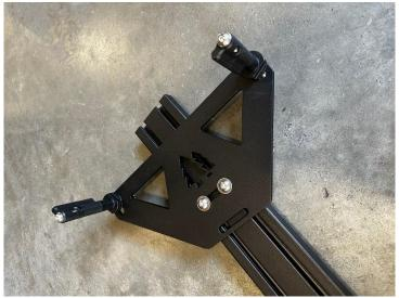
5. Align the 2 brackets so that the MaxTrax posts are 35 inches apart, and test fit your MaxTrax before tightening the bolts down.
