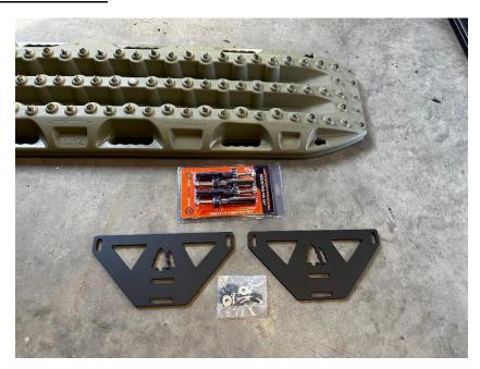
1. Mount your MaxTrax posts to the Greenlane brackets provided. Note that the MaxTrax posts are not included with the MaxTrax mounting kit and must be purchased from MaxTrax.
