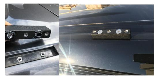
3. Fasten the 1/4" spacers provided to the bottom of the front rack tabs on the side panels. The 4 gutter blocks are the same height, but the spacers are required in the front to allow the rack to sit level. The spacer is threaded and can be attached with a 5/8" bolt and washer from the top side, as shown below. Install this loosely for now as some adjustment may be required in the next step.
