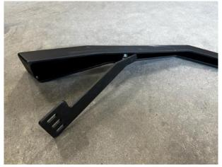
12. Remove the 3 factory bolts (per side) holding the stump bumper in place these will be replaced with the longer supplied bolts.
