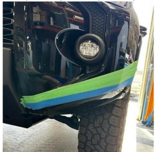
3. Trim the portion next to the bumper to expose the sides of the bumper – Do not cut higher than the corner point of the bumper yet.
