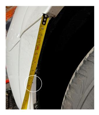
9. Hold up the wing and mark the areas where more cutting is required. Repeat this step until you have an even line with roughly ¼" gap between the wing and the bumper – Take your time and work up to the final cut line, you can always cut more but you can't add material back on!
