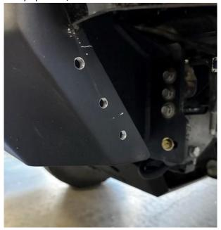
8. Mark your cut line with a sharple on the masking tape. The final cut measures 7.5" from the corner of the bumper, as shown. We recommend cutting around 1" below the final cut line to start.
