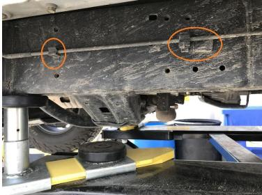
3. Unbolt the XREAS unit from the passenger and drivers side and remove the frame tab so the module can be reinstalled on top of the slider frame plate.
