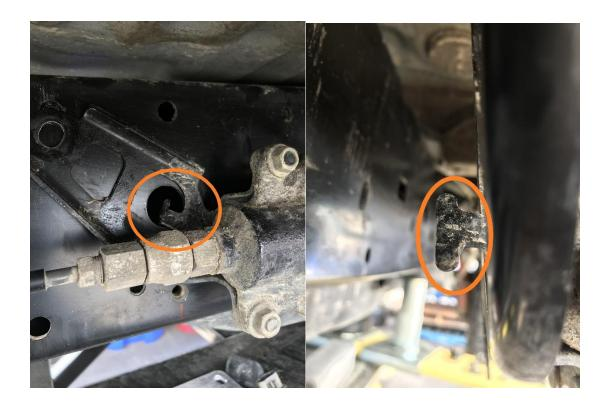
4. Remove parking brake cable bracket from frame – this bracket will be reinstalled on top of the slider frame plate.
