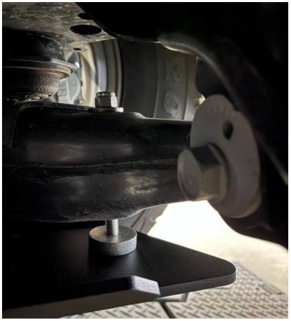
7. With each of the 3 bolts installed, tighten them evenly until each is hand-tight, and the control arm skid plate is fixed in position.
