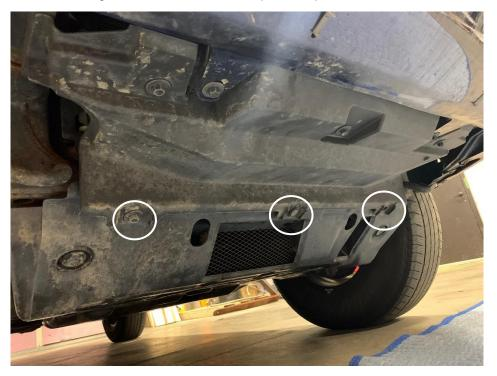
2. Remove factory skid plates by removing the 4 bolts from the front skid plate, and 4 bolts from the rear skid plate if applicable, using a 12mm socket (13mm socket if you have aftermarket hardware from a differential drop kit. You will not reuse this hardware OR the ½" spacers from the drop kit if applicable.
