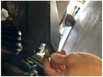
6. Lastly, install the 4" long 3/8" bolt through the rear-most hole with a 3/8" spacer between the skid plate and the control arm. Loosely install the washer and nylock nut on top of the control arm.
