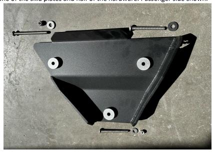
4. Starting with the 3" long 3/8" bolt, install it upwards into the front hole (closest to front bumper) with a 3/8" spacer between the skid plate and the control arm. Loosely install the washer and nylock nut on top of the control arm.
