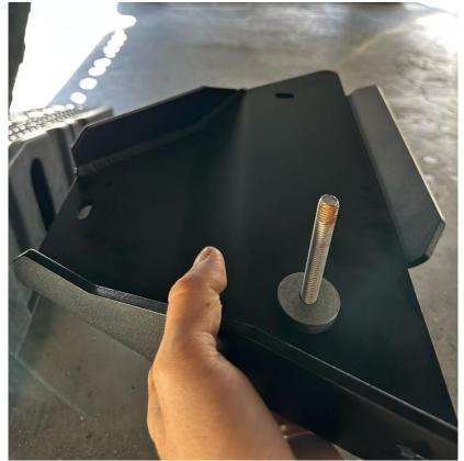
5. Next install the smaller 5/16" bolt in the smaller hole closest to the wheel with a 3/8" spacer between the skid plate and the control arm. Again, loosely install the washer and nylock nut on top of the control arm.
